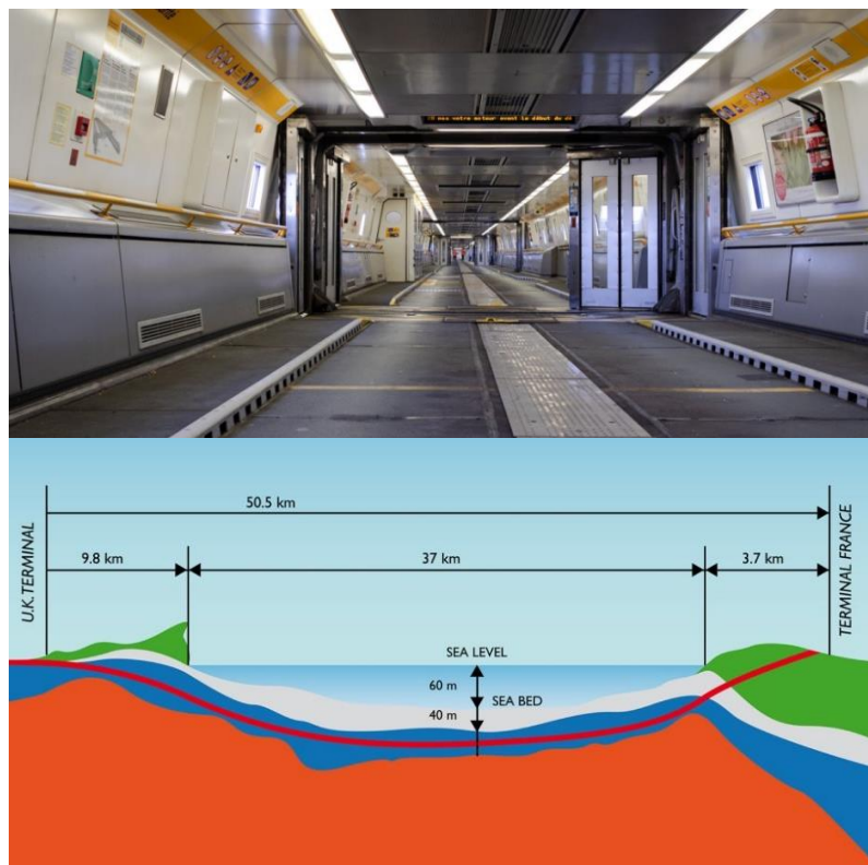
Figure 3-7: Cross section and longitudinal profile of Channel Tunnel
