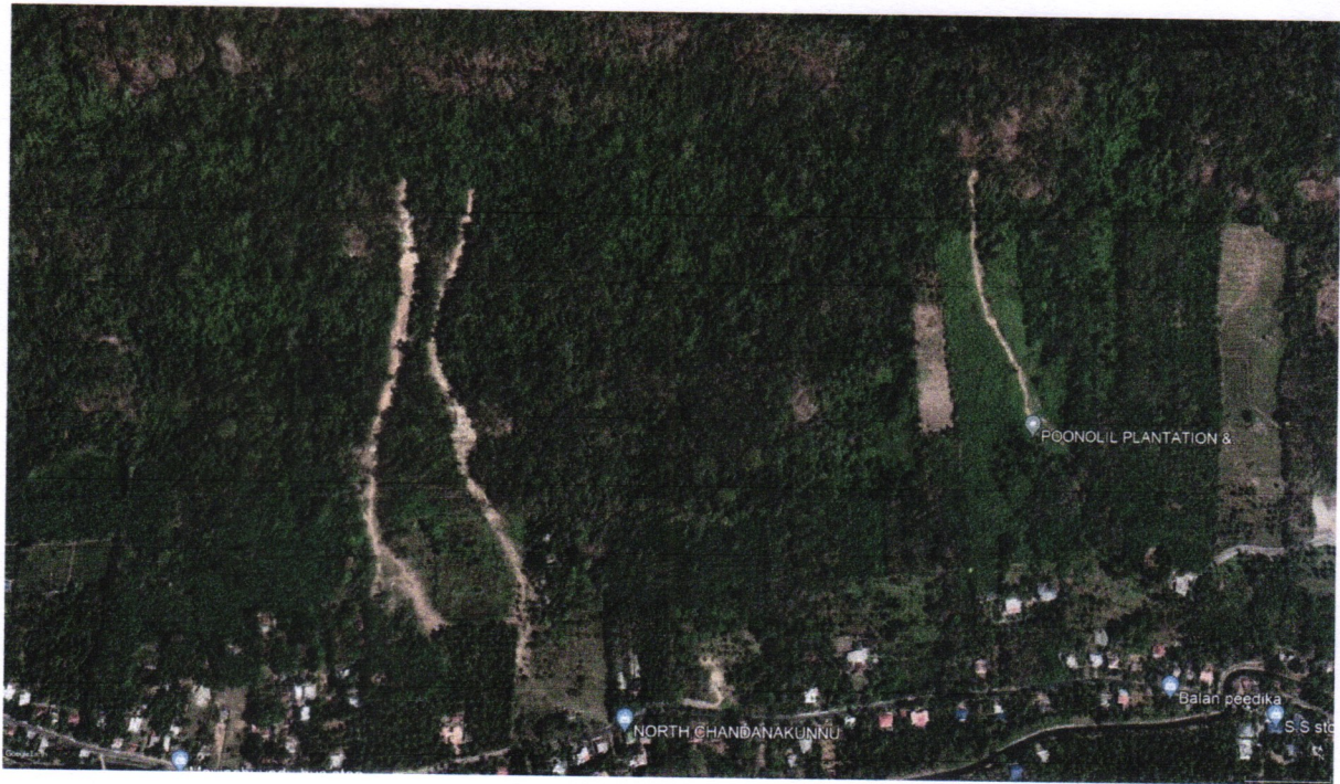
Fig. 5 High-resolution Google Earth image showing the three landslides that occurred in this panchayat. Note the long runouts that end just beneath the foothills
